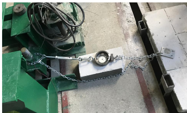
Fig.4 View of experimental stand for shear loading.
