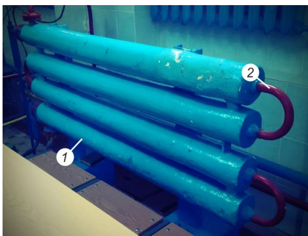
Fig.1. The laboratory «pipe-in-pipe» heat exchanger installation: 1 – the pipe for the cool agent, 2 – the pipe for a heat agent.
