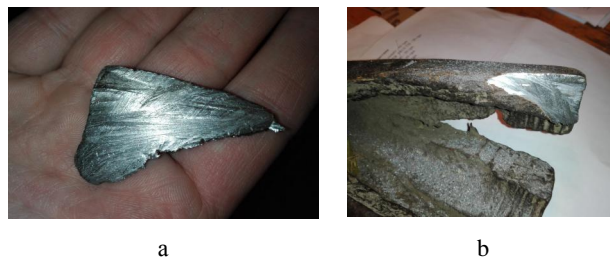
Picture 1. Specimen selection for microstructural analysis: a – blank for the specimen; b – destroyed breeching part of the destroyed cannon
