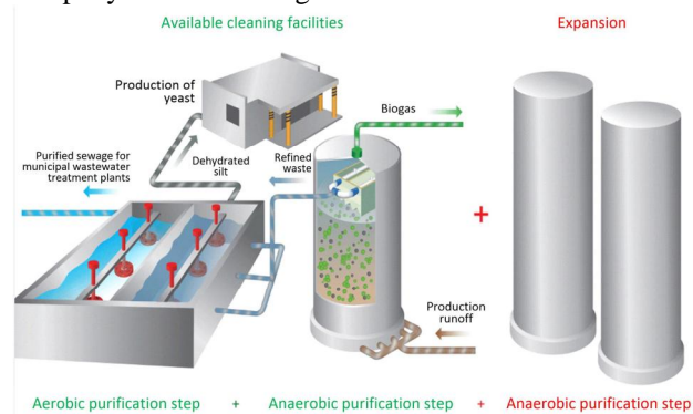
Fig. 2. Expansion scheme of the biogas plant of the company.
