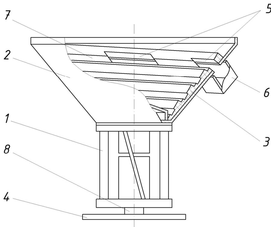
*Fig. 1. The design diagram of the vibratory separator*
