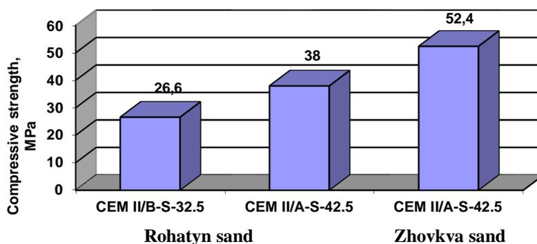
Fig. 1. Results of compressive strength test after heat treatment of fine-grained concretes (PC:S:BS=1:1.2:0.69)
