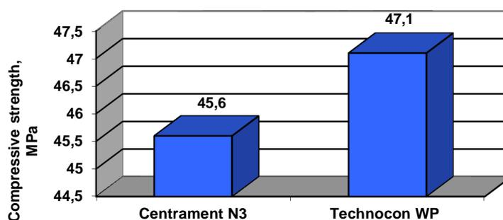
Fig. 2. Compressive strength of concretes after heat treatment
