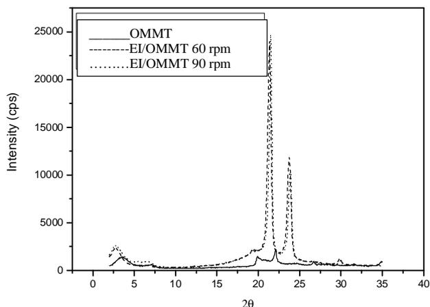
**Fig 1.** XRD patterns of OMMT (ss); EI/OMMT nanocomposites processed at 60 (—) and EI/OMMT nanocomposites processed at 90 rpm (.....)
