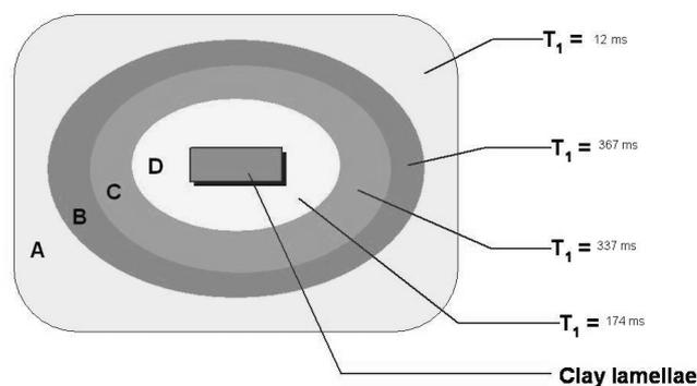
**Fig. 2.** Diagram of domain ordination in the formed nanocomposite
