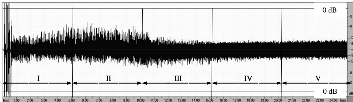
**Fig. 1.** Oscillogram of acoustic signal of the cavitation field generated by the magnetostrictive oscillator. Emitter capacity (W) changed with time (min): 8.0 (I); 9.2 (II); 10.2 (III); 11.5 (IV) and 12.5 (V)
