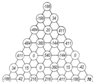
Fig. 7. Difference analogue of biharmonic operator  $27/4h^4\nabla^4$  for the 26-th node
