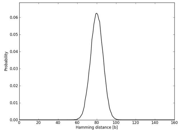
Fig. 3. Probability distribution of selecting the keys with the specified Hamming distances from any fixed key  $K$ .
