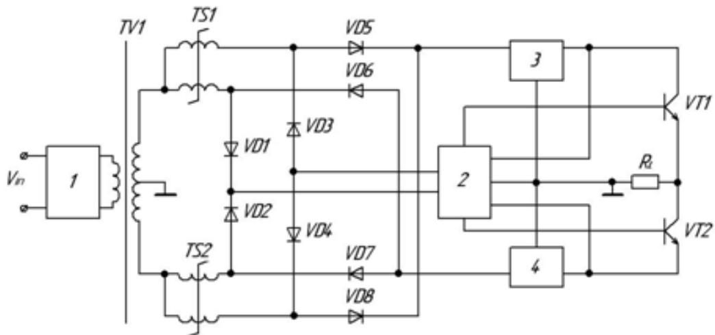
Fig. 7. Improved functional diagram of proposed high-frequency MagAmp inverter
