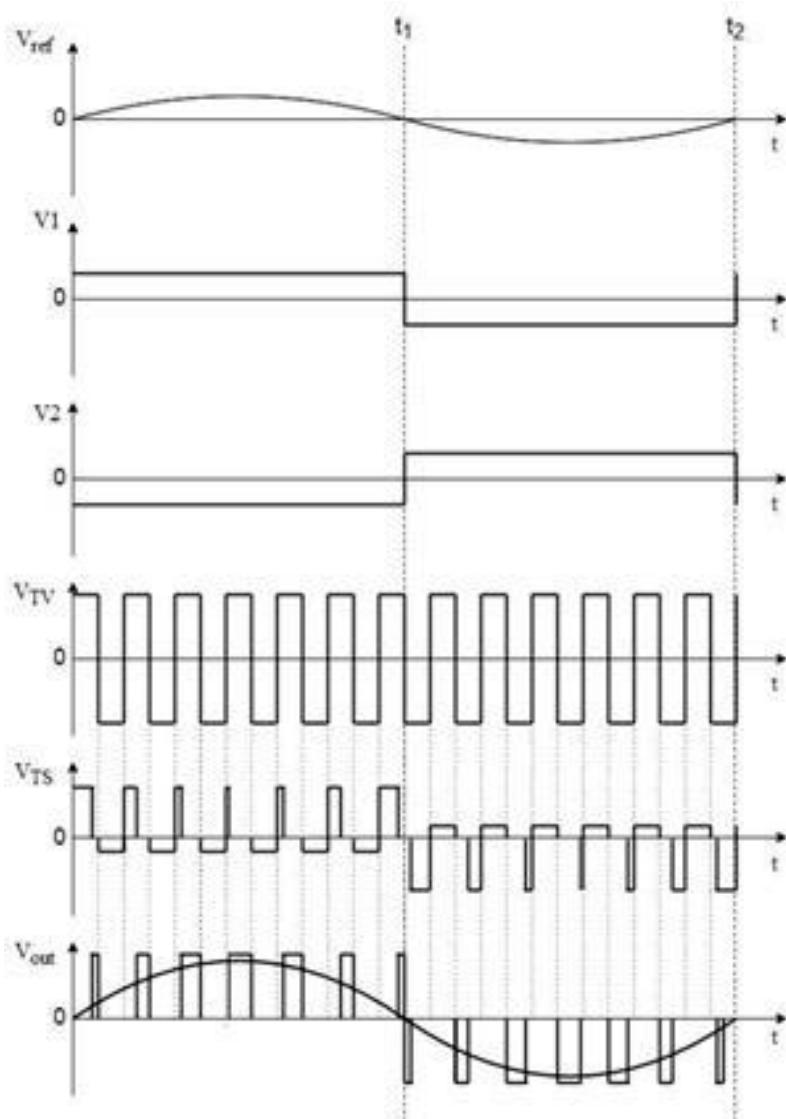
Fig. 8. Theoretical waveforms of MagAmp inverter.
