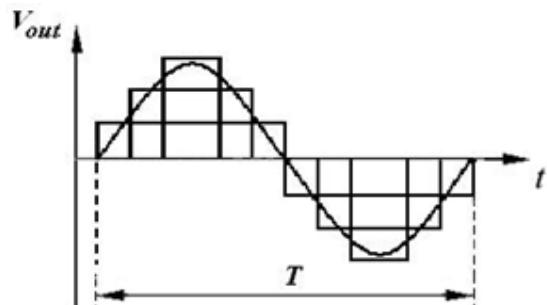
Fig. 1. Forming the output ac voltage at multilevel dc voltage commutation.
