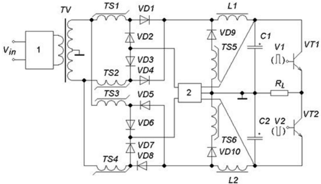
Fig. 6. Proposed circuit diagram of MagAmp Power Inverter
