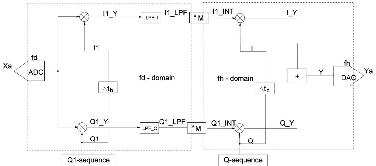
Fig. 3. Block diagram of Weaver's method of SSB modulation.
