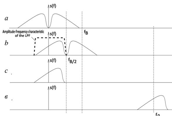
Fig. 2. Spectrum transformations in Weaver's SSB modulator.
