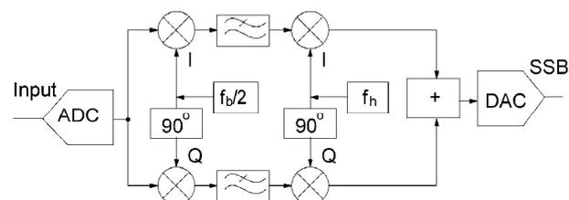
Fig. 1. Block diagram of Weaver's method of SSB modulation.
