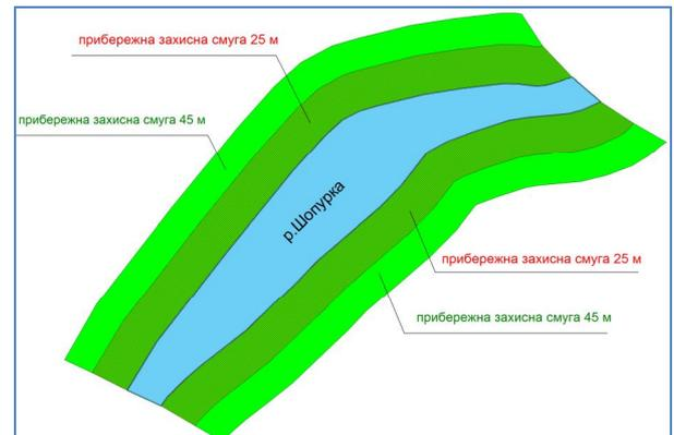
Fig. 6. Joint diagram of protective riparian zones along the r. Shopurka (part)
