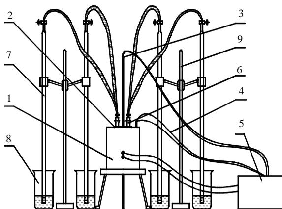
**Fig. 1.** Laboratory setup to determine coal inflammation temperature: electric furnace (1); copper block (2); thermocouples (3, 4); furnace temperature regulator (5); test tubes (6); burettes (7); glasses (8); laboratory supports (9)
