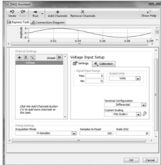
Figure 3. Configuring the device with help of DAQ Assistant
