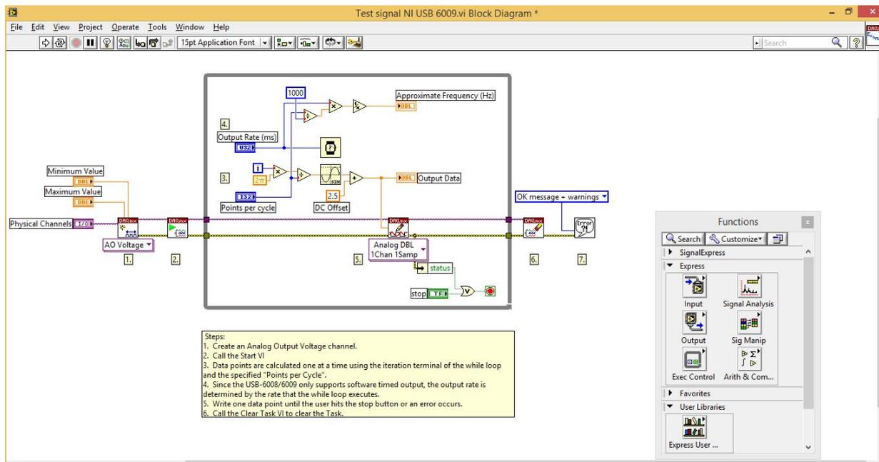
Figure 5. Block diagram of created virtual device
