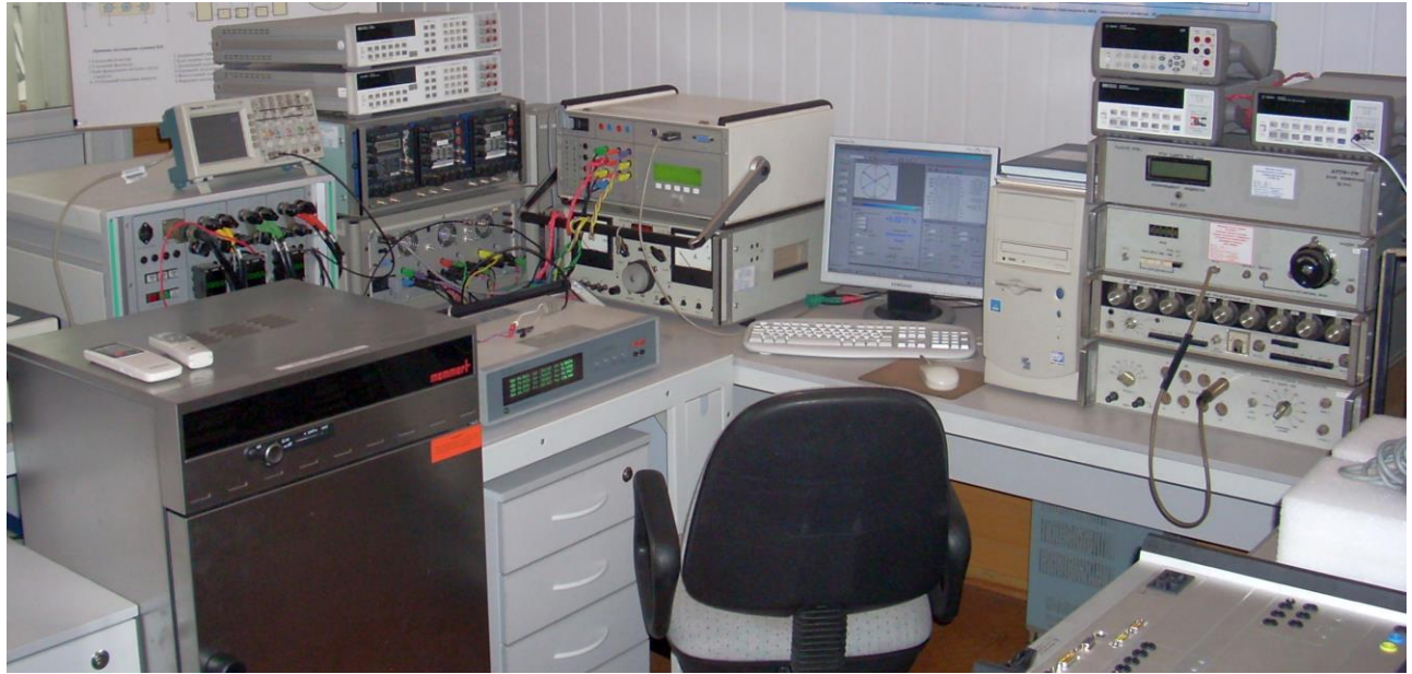
Fig. 2. Appearance of the National Standard of Ukraine for Units of Electric Power and Power Factor NDETU EM-08-2023
