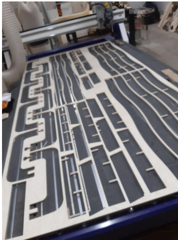
Fig. 3. Remains of multilayer plywood sheet after milling the bench frame
