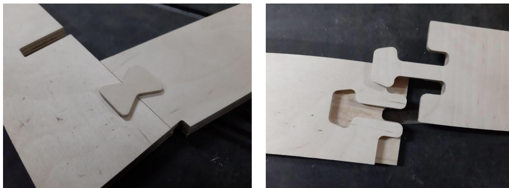
Fig. 1 a, b. Technological nodal joints are made on a CNC machine
