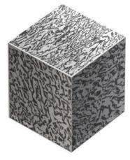
**Fig.1.** 3D view of the sample cut from YAG:Ce-Al<sub>2</sub>O<sub>3</sub> eutectic crystal
