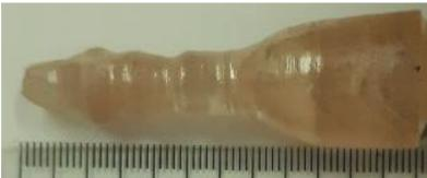
Fig. 1. Single crystal of Y<sub>0.85</sub>Gd<sub>0.15</sub>AlO<sub>3</sub>: 0.05 at% Mn, 0.5 at% Hf grown by the Czochralski method.
