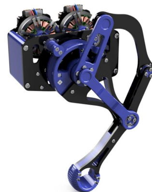
Fig. 1. 3D model of the designed leg
