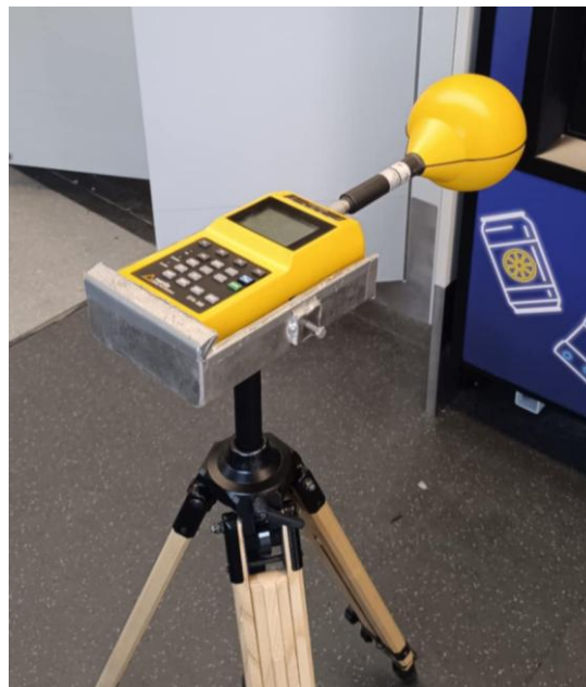
Research equipment – AC Field Analyzer
