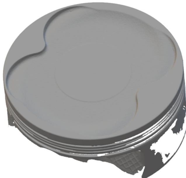
Fig. 1. 3D scans of a piston.
