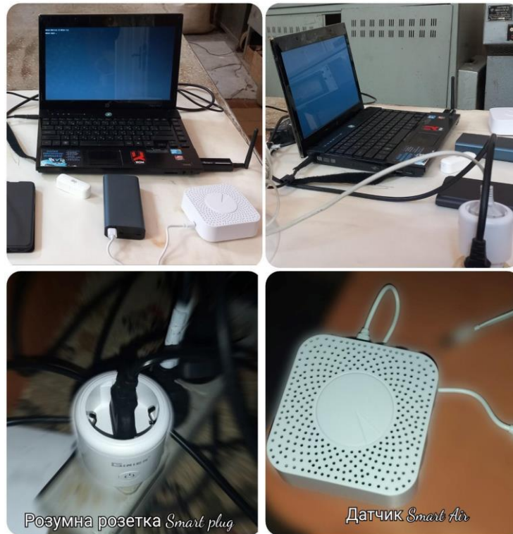
Fig. 1. Prototype of the air quality monitoring system in shelters based on the Internet of Things technology and the Home Assistant software package
