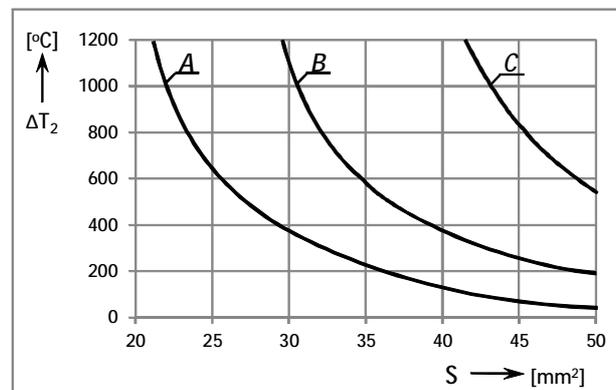
Fig. 2. Relationship between temperature rise  $\Delta T_2$  of air termination conductors and their cross-sectional area  $S$ , for three different values of specific energy of lightning discharge: A -  $0,5 \times 10^7\text{ A}^2 \cdot \text{s}$ , B -  $10^7\text{ A}^2 \cdot \text{s}$ , C -  $2 \times 10^7\text{ A}^2 \cdot \text{s}$ .
