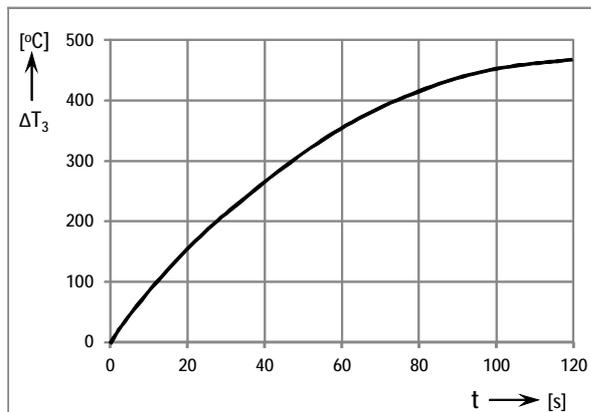
Fig. 5. Relationship between drop  $\Delta T_3$  of temperature rise  $\Delta T_2 = 500^\circ\text{C}$  and time  $t$ , during cooling down of air termination conductor model.
