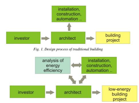
Fig. 2. Design process of low-energy building
