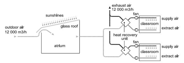
Fig. 3. Mechanical ventilation with heat recovery system and preheating of supply air in atrium
