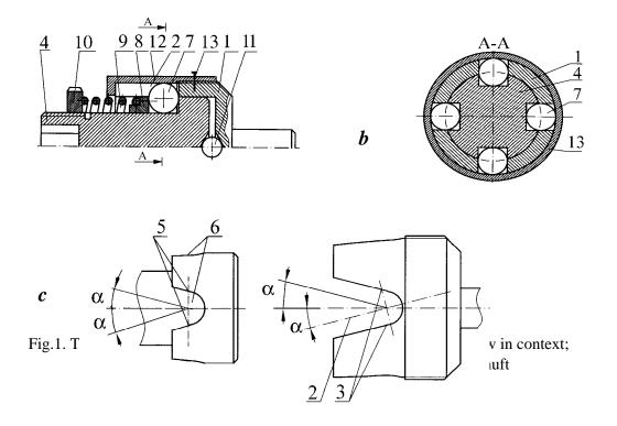
The structure of the torque limiter or tightening force nuts narizevyh connections has: driving pivmuftu 1 of grooves 2, with two sloping surfaces 3; driven pivmuftu 4 of grooves 5 which are also inclined surfaces 6 under the same angle as the in the leading pivmufti; balls 7, located both in the grooves of driving and driven pivmuft; screw drive 8, which nestles on the balls spring 9; adjusting nut 10, the ball 11 for centering, housing 12 with screws 13 for fixing it.
