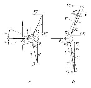
Fig. 2. Power interaction between the ball and side surfaces of the grooves pivmuft during off coupling: a - friction is not included, b - considering friction
