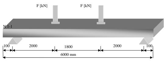
Fig. 2. Static scheme supported beam
