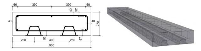
Fig. 1. Size and shape of beam N1
