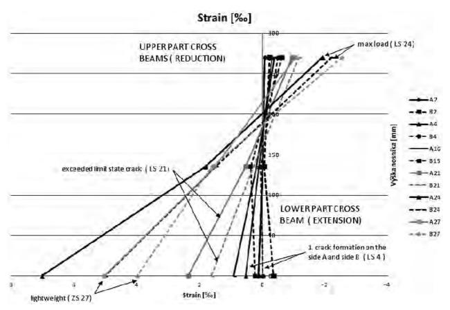
Fig. 6. Graphical representation of strain during the height of the beam
