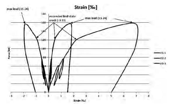
Fig. 5. Graphical dependence of strain and force during loading
