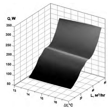
Fig. 4. Dependence the power of thermosyphon heliocollector, Q, W, from the temperature difference of cold air in the experimental modules and heated air after heliocollector,  $\Delta t$ , ° C, and it's volumetric flow rate, L, m<sup>3</sup>/hr
