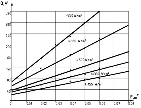
*Fig. 3. Dependence the power of thermosyphon solar collector, Q, W, changes in the area of inlet and outlet of heliocollector, F, m<sup>2</sup>, and the intensity of heat flow, I, W/m<sup>2</sup>*
