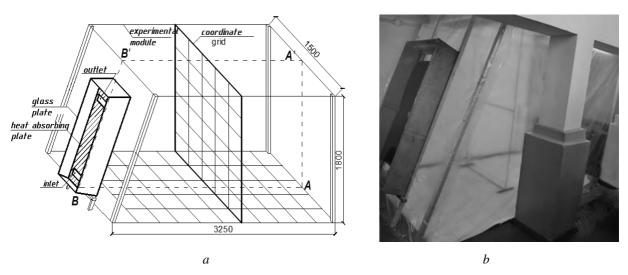
Fig. 2. Scheme (a) and photo (b) of experimental module
