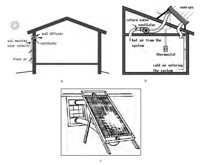
Fig. 1. Options for installation of solar air heaters: on the wall, b) on the roof, c) in the yard
