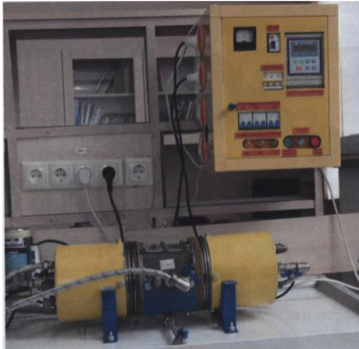
Fig. 1. Electromagnetic cavitator for cavitation treatment of chemically active substances of liquids, liquids under pressure and at the promoted temperatures (with the partly taken off protective elements of sheepskin coat)
