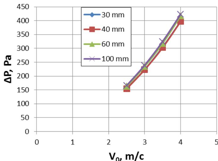
Rice. 1. Dependence of hydraulic resistance of vehicle is on fictitious speed at the different values of number of coils (the width of the entrance union coupling for all vehicles is evened a 60 mm)
