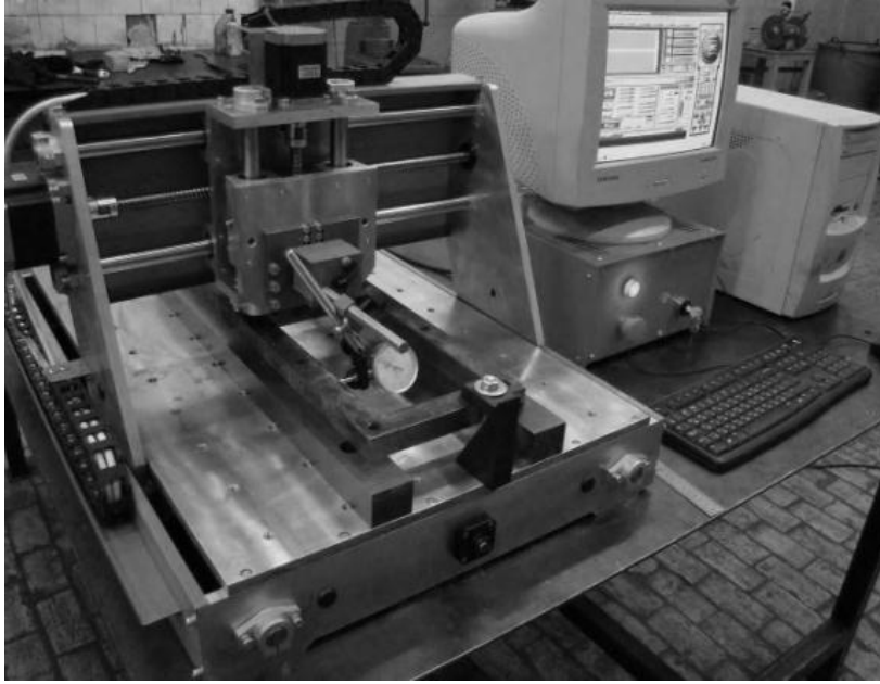
Fig. 2. Measuring system during scanning of the die working surface
