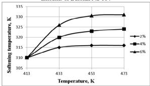
**Fig. 4.** Softening temperature *vs* preparation temperature at different amounts of Butonal NS 104
