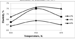
**Fig. 6.** Bitumen elasticity *vs* preparation temperature at different amounts of Butonal NS 104
