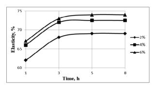
**Fig. 5.** Bitumen elasticity *vs* preparation time at different amounts of Butonal NS 104
