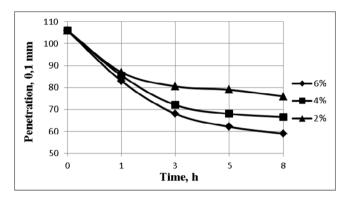
**Fig. 1.** Bitumen penetration at 298 K *vs* preparation time at different amounts of Butonal NS 104
