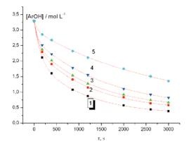
Fig. 3. Kinetic curves of ArOH consumption in the catalytic reaction with methyl acrylate in the presence of the ArOK monomer in DMSO (1), DMF (2), HMPA (3), DME (4),
