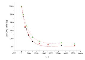
Fig. 1. Kinetic curves of the reaction of ArOH with methylacrylate (MA) in the presence of the ArOK monomer at 398 (1), 389 (2), and 378 (3) K;  $[ArOH]_0 = 3.29 \text{ mol} \cdot l^{-1}$ ,
