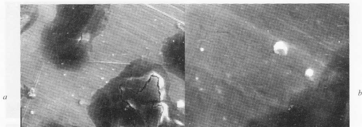
Fig. 6. Pictures of precipitated (5 mass %) solution of PEG2000 in CON: \times 600 (a), \times 4000 (b)
