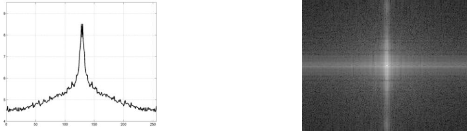
Fig. 10. Visualization of discrete Fourier transform results for the image with natural blur
