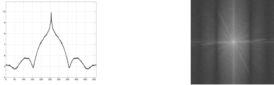
Fig. 7. Visualization of discrete Fourier transform results for the image with artificial horizontal blur of 5 pixels
