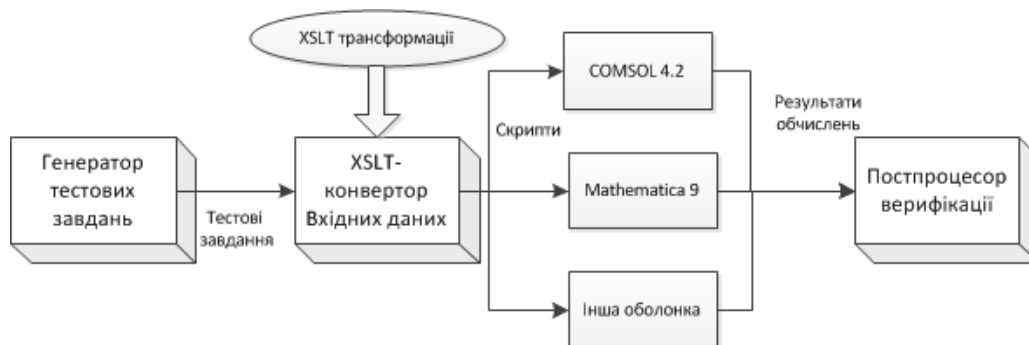
Fig.1. Core software architecture for testing and verification problem solving methods of mathematical physics problems
