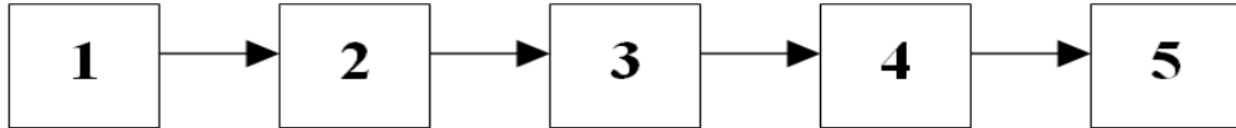
Fig.1. The structural scheme of the experiment for the selection of PV signal: 1 - source of UV radiation; 2 - a sample of material; 3 - measuring transducer, 4 - digital oscilloscope; 5 - computer
