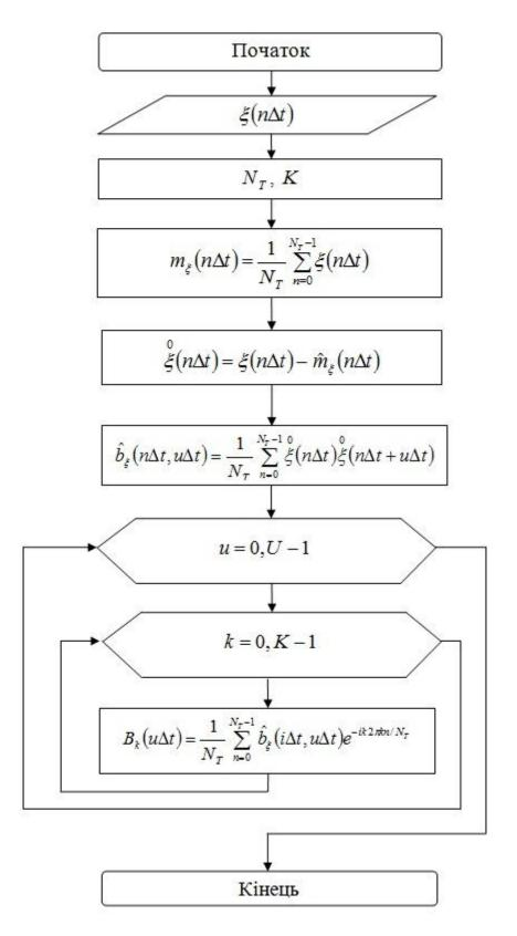
Figure 1. Block diagram EGS component method processing
