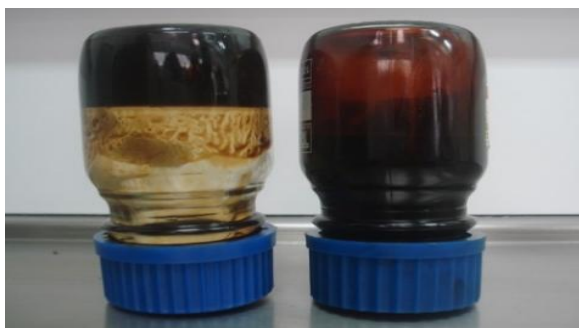
Fig. 6. The effect of Mic- (at the left) and Mac-wax (at the right) on the flowing properties of crude oil used in the study
