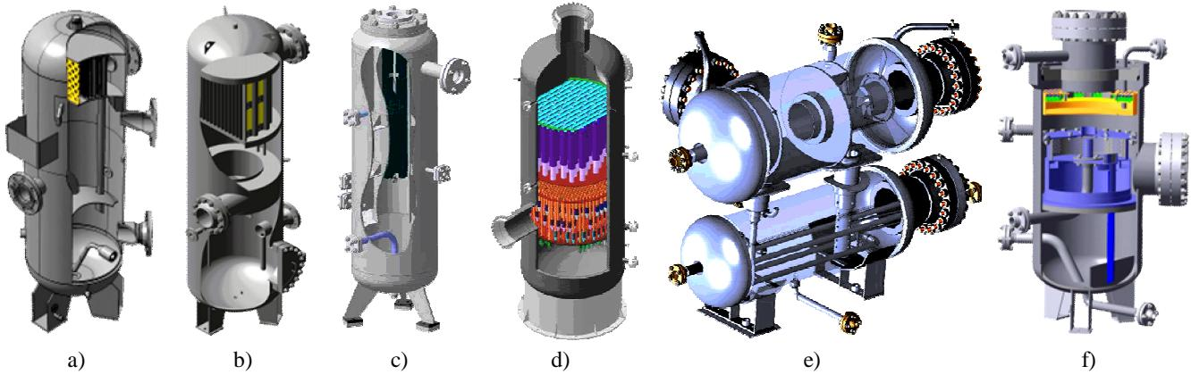
**Fig. 1.** 3D model of highly effective gas separators: louvre separator of the inertial type (a); louvre separator of the filter inertial type (b); vortex separator with the cartridge filter (c); separator for natural gas thin cleaning with centrifugal elements and the section of mist elimination (d); block inertial gas-dynamic separator with vortex and louvre blocks (e) and a mass transfer counter-vortex separation device for natural gas dehydration
