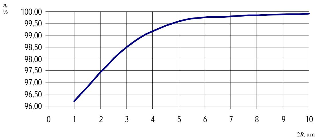
**Fig. 4.** Trapping efficiency at the 2<sup>nd</sup> stage of separation (filter-coalescer)
