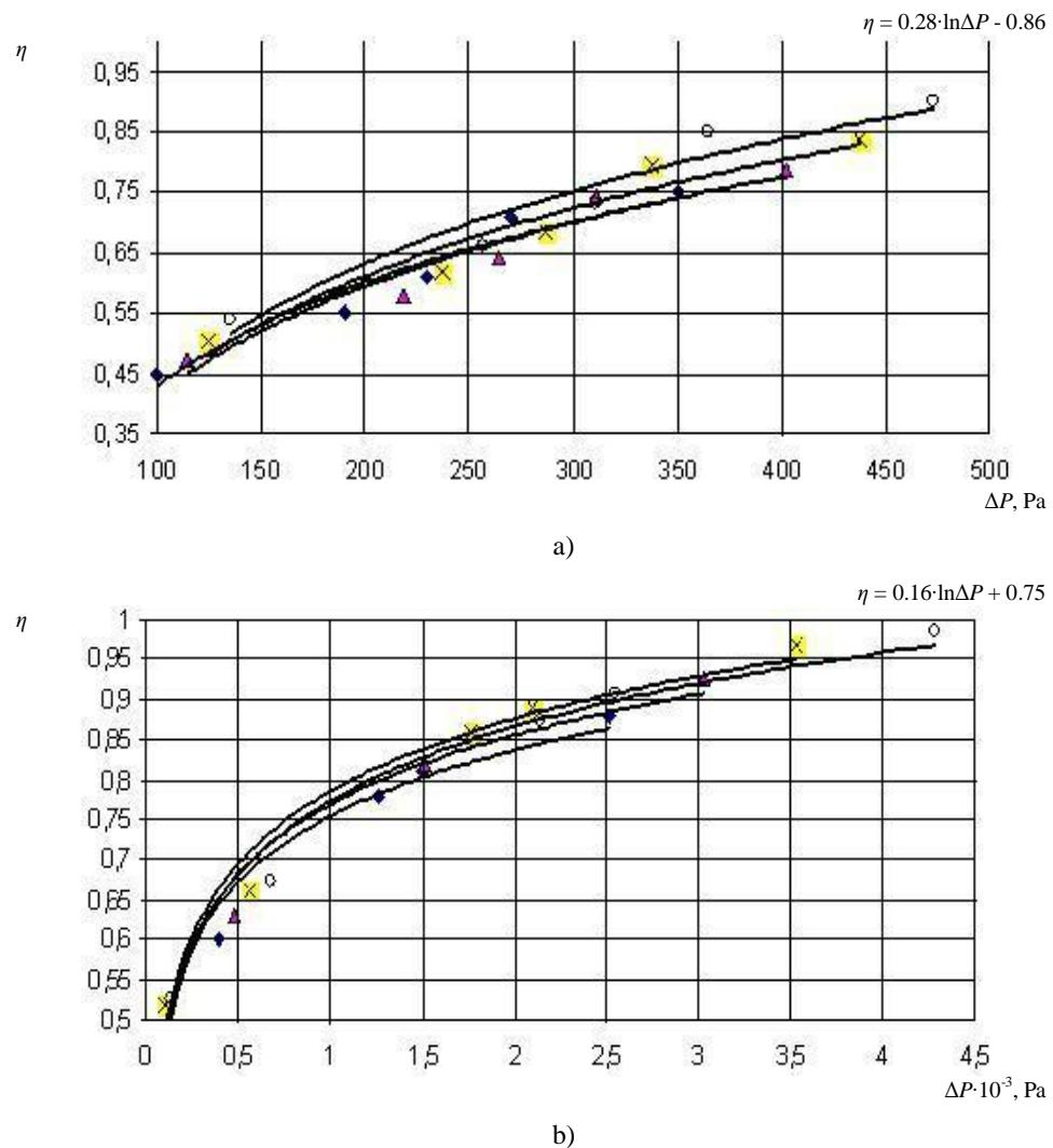
**Fig. 7.** Dependence of entrapping efficiency on hydraulic resistance of drop catcher (a) and mist eliminator (b): ■ –  $F/G = 0$ ; ◆ –  $F/G = 0.05$ ; ▲ –  $F/G = 0.10$ ;
