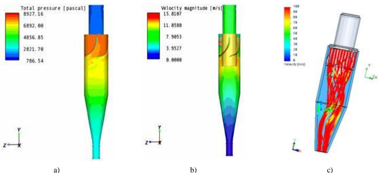
**Fig. 3.** Visualization of computer experiments: pressure difference on a cyclone wall (a); local velocities of gas flow along cyclone longitudinal section (b) and visualization of flow structure (particles motion path) (c)
