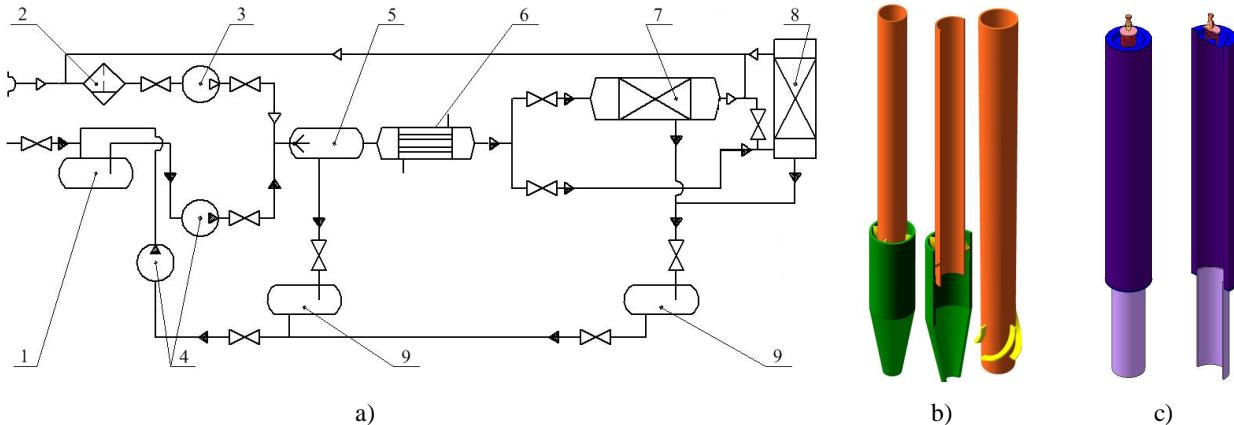
**Fig. 2.** Experimental plant for hydrodynamics investigation during separation of two-phase flows: experimental stand (a); drop catcher (inertial cyclone element) (b) and mist eliminator (filter-coalescer) (c). For experimental stand (a): vessel (1, 9); filter-drier (2); blower (3); pump (4); mixing chamber (5); heat exchanger (6); 1<sup>st</sup> stage of separation, drop catcher (7) and 2<sup>nd</sup> stage of separation, mist eliminator (8)
