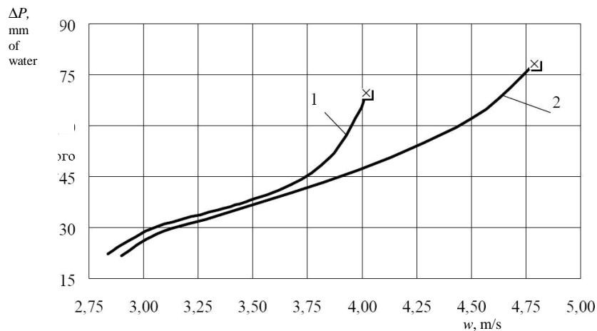
**Fig. 5.** Dependence of hydraulic resistance on gas flow velocity: gravity-inertial separator (1) and inertial filtering drop catcher (2). Critical point of phase inversion (X) corresponds to the flood mode
