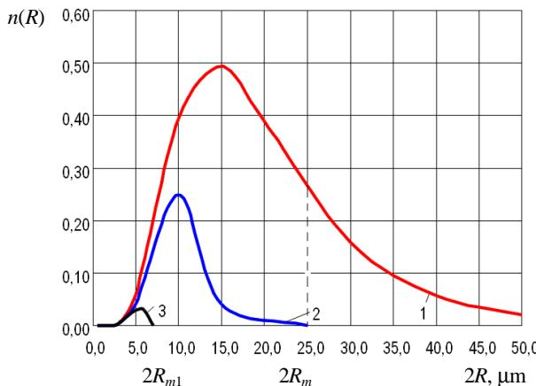
**Fig. 8.** The distribution of solid particles and fluid drops by size in the natural gas flow which are trapped by the first and second separation stages of device: distribution of the particles in the flow at the device inlet (first stage – battery block of cyclone unit) (1); distribution of the particles in the flow at the inlet to the second stage (block of cartridge filter-coalescer) (2) and residual distribution of the particles in the flow at the device outlet
