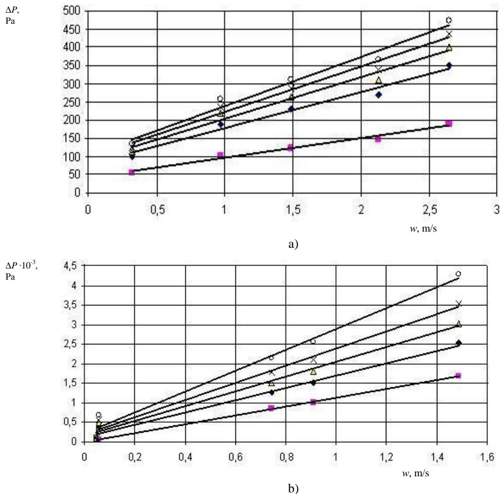
**Fig. 6.** Dependence of hydraulic resistance of drop catcher (a) and mist eliminator (b) on unit rate of trapped fluid at gas and aerosol movement: ■ –  $F/G = 0$ ; ◆ –  $F/G = 0.05$ ; ▲ –  $F/G = 0.10$ ; ✕ –  $F/G = 0.15$ ; ○ –  $F/G = 0.20$
