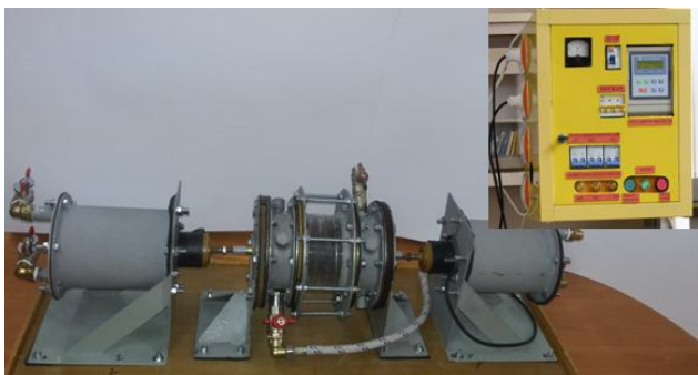
Fig. 2. Photo of experimental low-frequency electromagnetic vibration cavitator of resonance action for BW treatment
