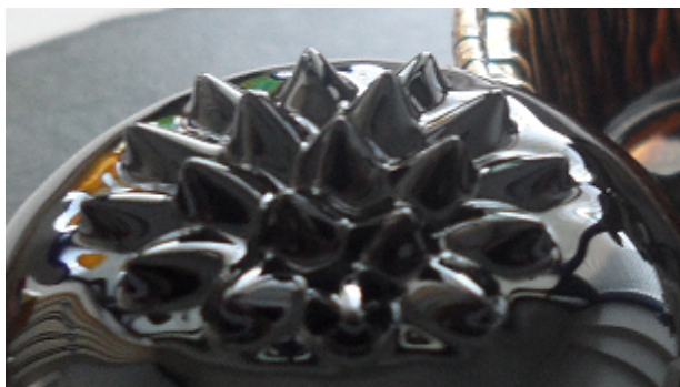
Fig. 1. Typical structure of magnetic fluid under the influence of external magnetic field.
