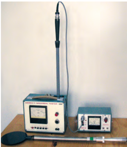
Fig. 2. MEH-type meter tested using the USMEH-type tester.
