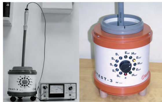
Fig. 4. MEH-type meter tested in UTEST-3 type tester.
