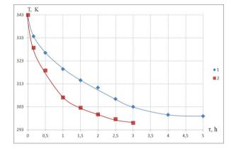
**Fig. 3.** Suspension temperature *vs.* bubbling time: air temperature 297 Kand humidity 65 % (1); air temperature 283 K and humidity 88 % (2)
