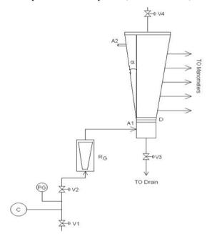
**Fig. 1.** Schematic diagram of experimental setup [2]: A1 - air inlet; A2 - air outlet; D - distributor; C - compressor; PG - pressure gauge;  $R_G - gas$  rotameter; V1 - V4 - control valves
