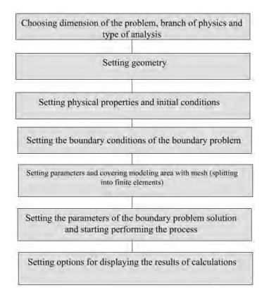
Fig. 2. An algorithm for constructing models in COMSOL
