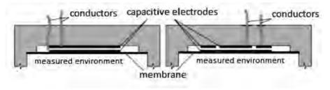
Fig. 1. The capacitive pressure sensor
