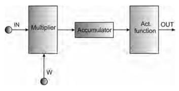
Fig. 3. Multiplier/accumulator architecture
