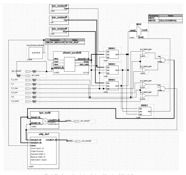
Fig.4. Hardware-description design of functional block diagram of discrete-time KWTA neural circuit presented in [21, 22]
