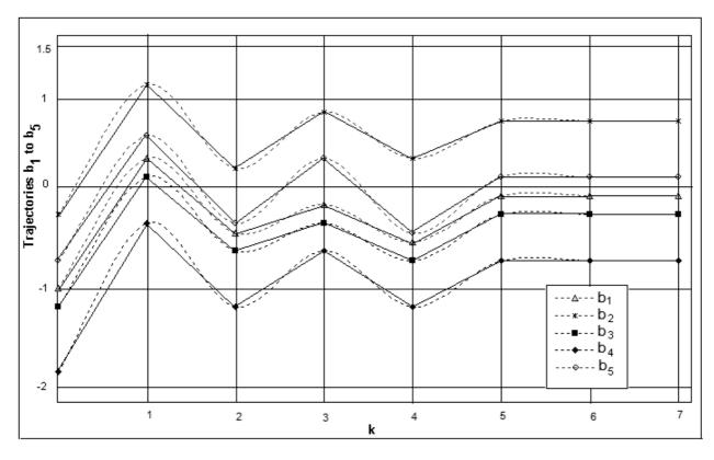
Fig. 5. The trajectories of the outputs  $b_i^{(k)}$ , i = 1,2,3,4,5 of the FPGA based hardware implementation of neural circuit presented in [21, 22]
