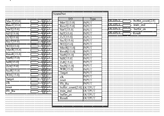
Fig. 2. Top entity for VHDL model of the network
