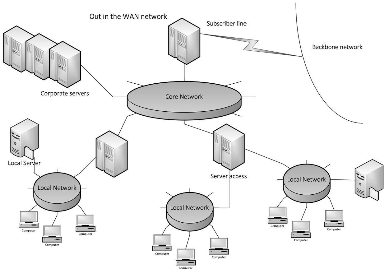
Fig. 2. The structure of corporate network CAD [1].
