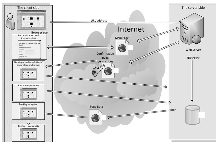
Fig. 7. Architecture of Web-oriented CAD
