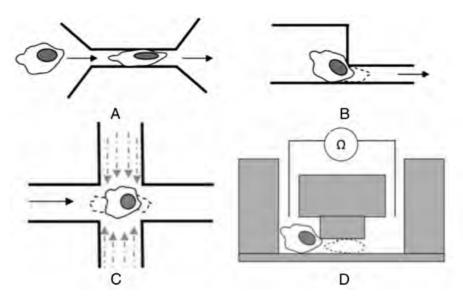
Fig. 2. Microfluidic manipulations (A) Constricted Geometry (B) Aspiration Induced (C) Fluid Induced (D) Electrically Induced
