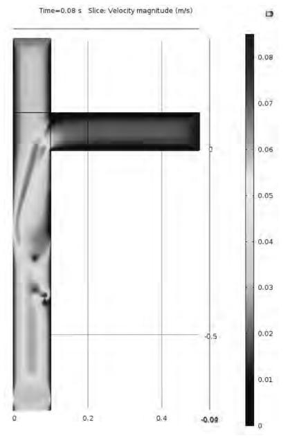
Fig. 7. Distribution of the velocities of fluid in the T-mixer
