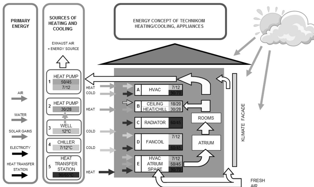
Fig. 2. Energy supply concept heating – cooling – ventilation
