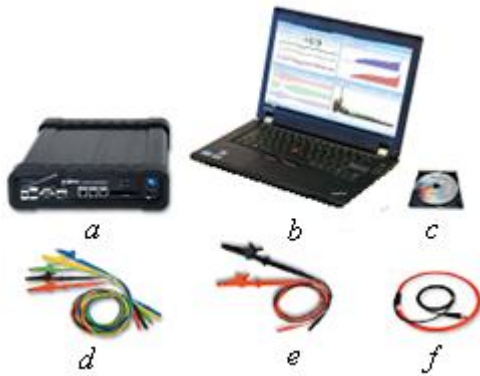
Fig. 1. A Set of instruments for measuring the dynamics parameters of electrical loads of household appliances: a – a portable device G4500 BLACKBOX Portable; b – a notebook for monitoring processes on the network; c – PQSCADA software; d – AC wires; e – DC wires; f – a flexible AC clamp meter.
