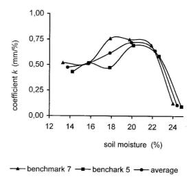
**Fig. 4.** Effect of absolute soil moisture on the value of the coefficient *k* at benchmarks 5 and 7.
