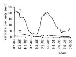
**Fig. 1.** Vertical movements at GTG in Poltava 2017 - 2018:
