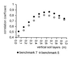
**Fig. 2.** Dependence of the correlation coefficients between the vertical movements at benchmarks 5 and 7 and the moisture of the soil layers with thickness 0.1 m in the depth range 0-1.0 m for the period 2006-2015.
